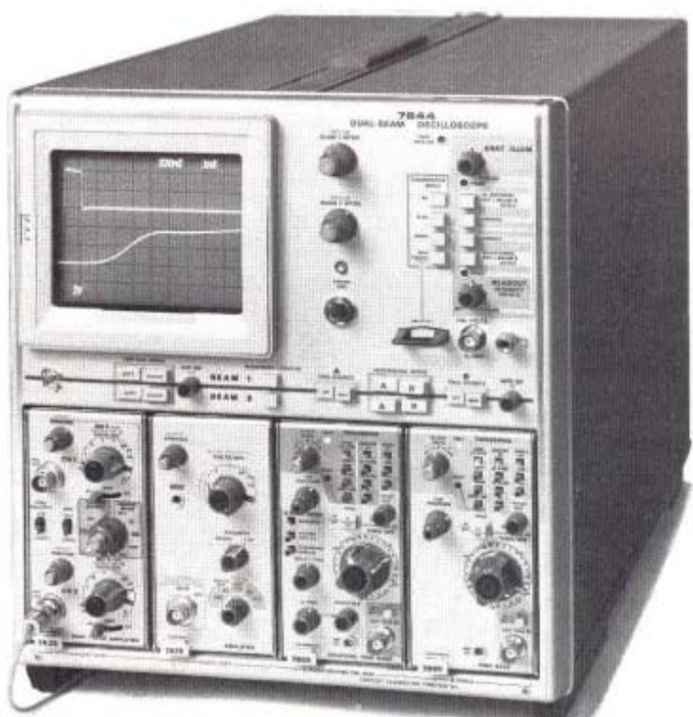
**Horizontal Separation** — Beam 1 can be positioned at least 0.25 cm to the right and at least 0.25 cm to the left of Beam 2 with a total 2 cm range.
